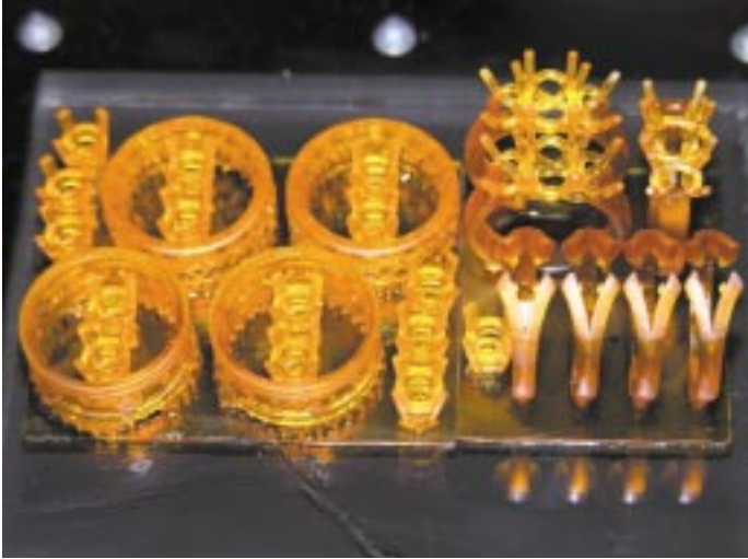
Left: 3D resin models built using digital light processing from Envisiontec
